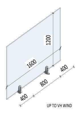
Client: STORETECH LIMITED Project: MILFORD FIXING SPIGOT Drawing: PANEL SIZES - POOL FENCE 1
