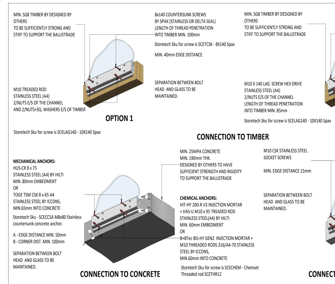
A - EDGE DISTANCE MIN. 50mm B - CORNER DIST. MIN. 100mm
